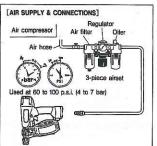
FITTINGS: Install a male plug on the tool which is free flowing and which will release air pressure from the tool when disconnected from the supply source.
