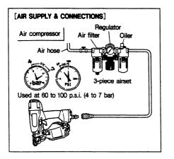
FITTINGS: Install a male plug on the tool which is free flowing and which will release air pressure from the tool when disconnected from the supply source.
