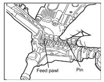
4 Push in the pin coil along the bridge until it has reached the end. Put the first pin into the hose.
