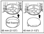
② When using 40 mm (1-1/2") nails, attach the nail support in such a manner that a mark "40" can been seen. When using 65 mm (2-1/2") ones, attach the nail support upside down.
