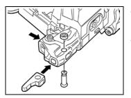
② Attach a new nail leg guide, set the pin and put back the rubber washer.
