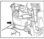
To detach, push the latch on the back of the magazine with a finger.
